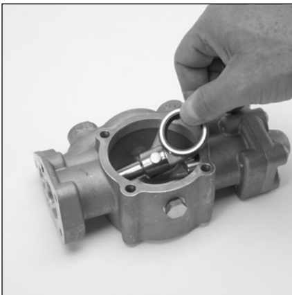
5.20 Remove and inspect connecting rod, plunger rod and wrist pin assembly.
