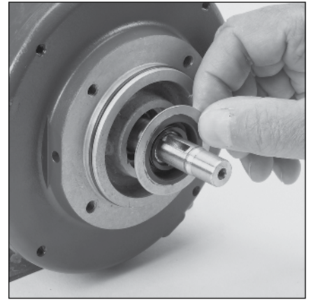
6.3 Lubricate and install shaft seal (10) with stainless steel flange facing out (towards pump).
