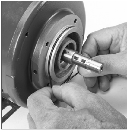
6.2 Lubricate and install motor flange o-ring (12) onto the motor flange.
