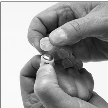
6.22 Place tapered side of seat (24) towards retainer (27) and snap into place.
