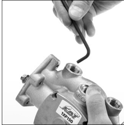
5.15 Insert the short end of an allen wrench to remove discharge valve assembly.
