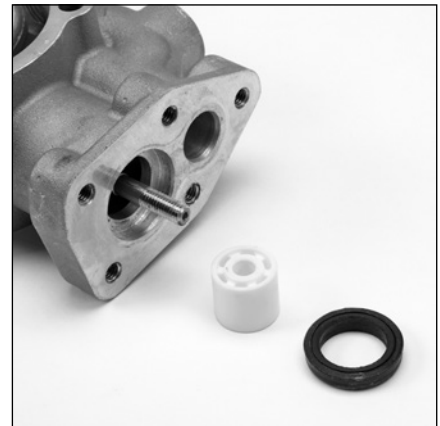
5.19 Remove and inspect ceramic plunger (21) and high pressure seal (22) from crankcase body (1).
