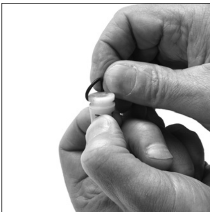
6.23 Lubricate and install o-ring (23) to seat (24). Repeat for second valve assembly.
