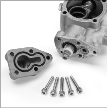
5.14 Use a 5mm allen wrench to remove five (5) M6x30 screws (13) holding head cover (14) to crankcase body.
