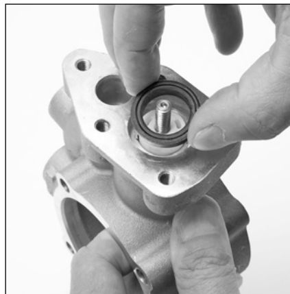
6.14 Lightly lubricate and install high pressure seal (22) with v-groove facing up over ceramic plunger (21).
