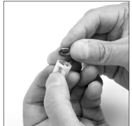
6.21 Place valve (25) cupped side over the spring (26).
