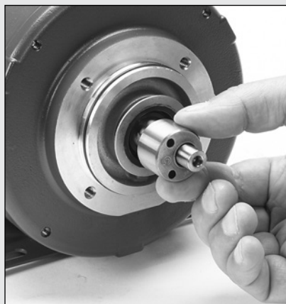
6.5 Hand thread cam (8) with stamped ID number and small holes facing pump (clockwise).
