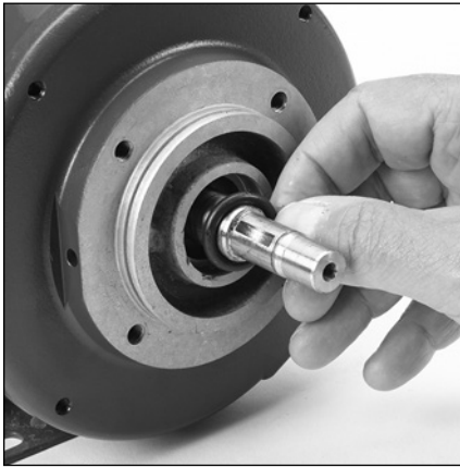
6.1 Lubricate and install slinger o-ring (11) into motor flange by sliding over motor shaft. Center between shaft seal bore and back of the slinger seal bore.
