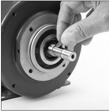
6.7 Lubricate and install woodruff key (9) into motor shaft keyway. (Keyed Shaft only).
