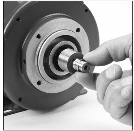
6.9 Install retaining ring (7) into snap ring groove on motor shaft to secure cam (8). (Keyed Shaft only).
