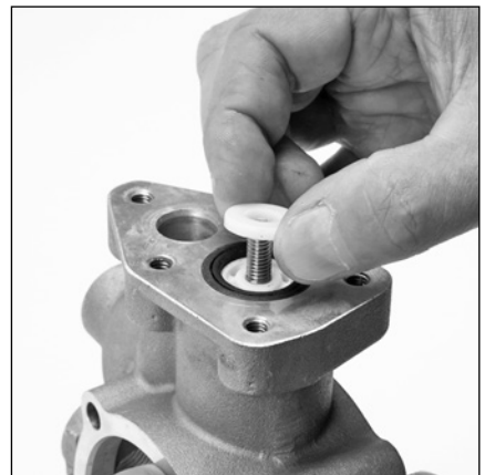
6.15 Install inlet valve (20) with flat side down onto plunger (21).
