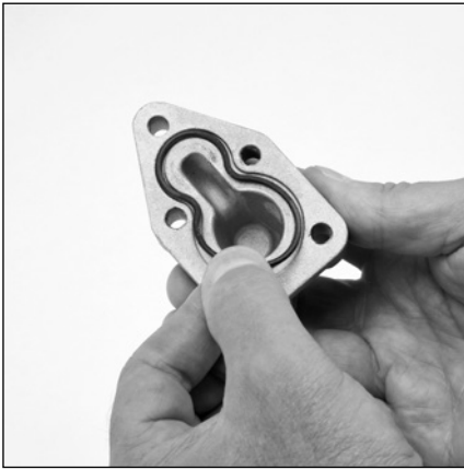
6.25 Lubricate and install o-ring (15) into head cover. Repeat for other cylinder head.
