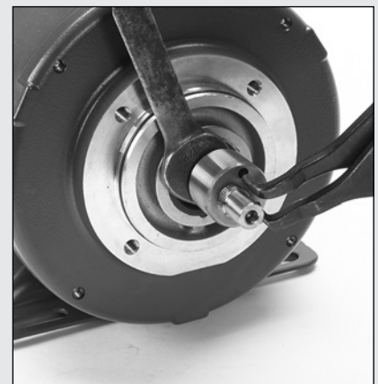
6.6 Use spanner wrench and 1/2" open wrench to tighten cam (8). NOTE: Apply Loctite® 242® to threads of motor shaft.
