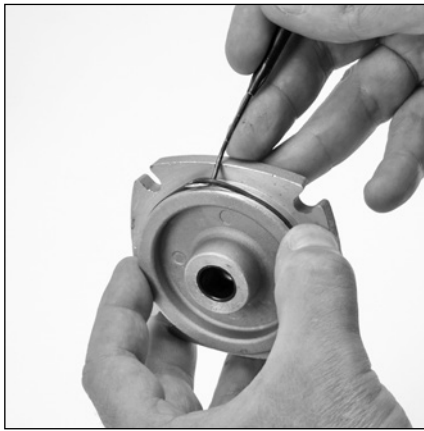
6.10 Lubricate and install o-ring (6) onto bearing cover (5).
